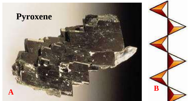
Figure 2-6 A) Black to green color of pyroxene mineral and B) Single-Chain Silicates
