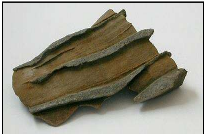
Figure 4-7 Shale is made up mostly of platy clays.
