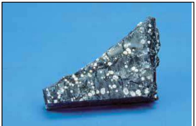
Figure 5-6 Hornfels forms by metamorphism of shale.
