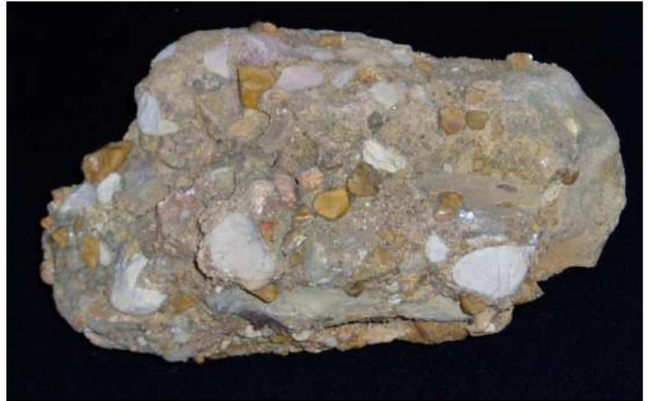
Figure 4-5 Poorly sorted and angular grains of Breccia
