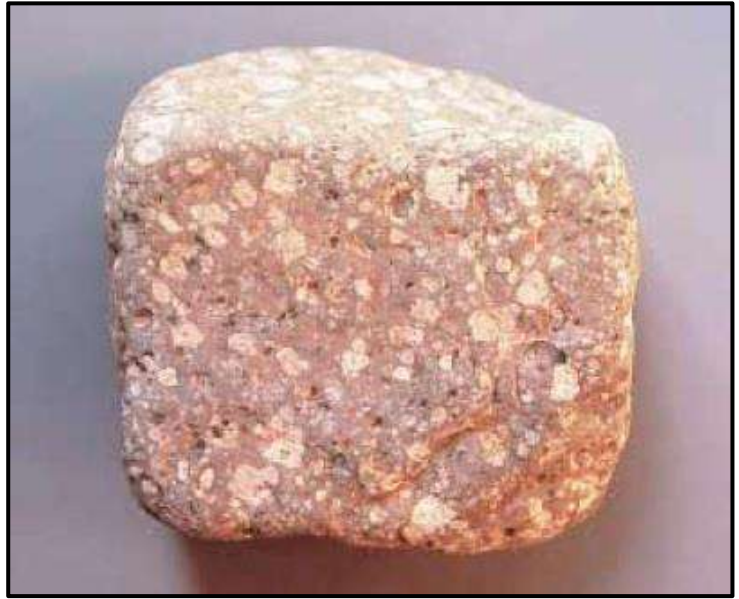
Figure 3-13 Porphyry is an igneous rock containing large crystals embedded in a fine-grained matrix. This rock is rhyolite porphyry with large pink feldspar phenocrysts.
