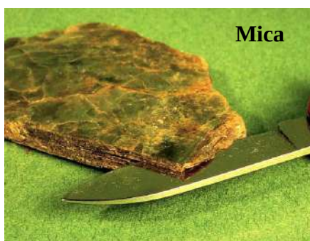
Figure 3-16 One set of cleavage in Mica mineral
