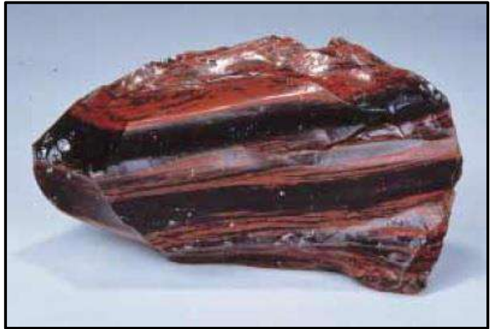
Figure 3-11 Obsidian is natural volcanic glass. It contains no crystals. (Geoffrey Sutton)
