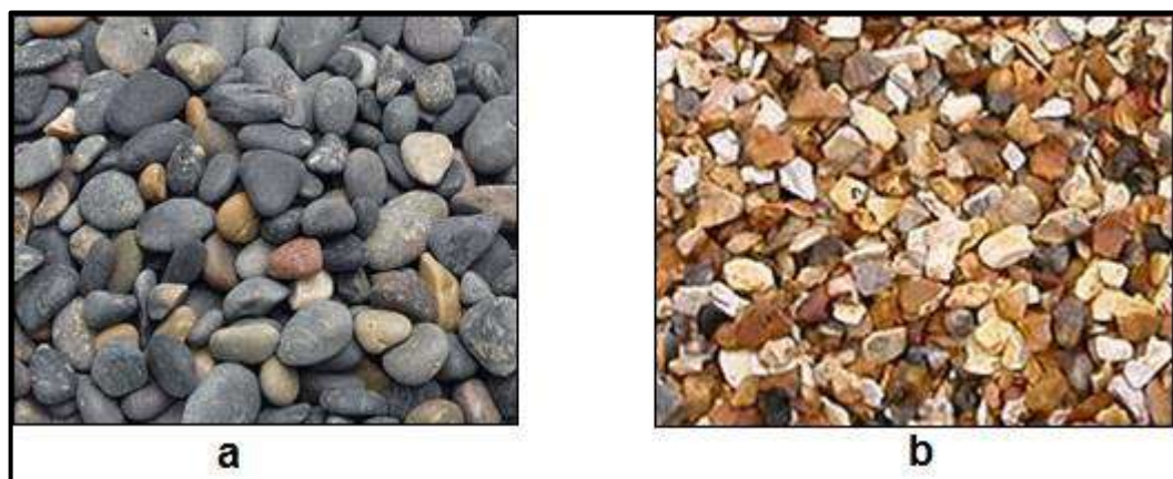
Figure 4-3 Well-rounded spheroidal grains (a) poorly rounded angular grains (b).
