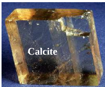
Figure 3-18 three sets of cleavage (at 90^\circ and oblique) in Halite and Calcite minerals.
